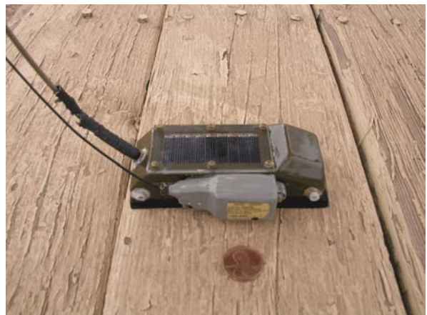
Figure 4. A 70 g GPS unit with a side-mounted VHF transmitter (gray) used to track bald eagles.
