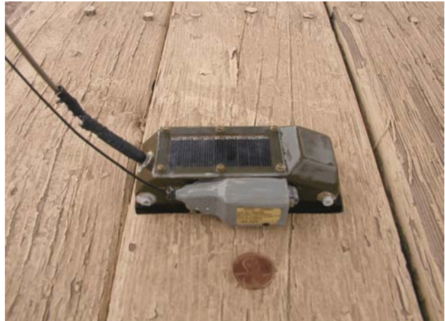
Figure 6. PTT GPS unit with VHF transmitter (gray) attached to the side. The whole unit weighs approximately 100 g.
