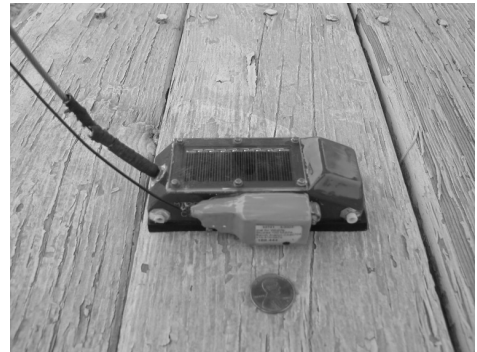
Figure 3. PTT GPS unit with VHF transmitter (gray) attached to the side. The whole unit weighs approximately 100 g.
